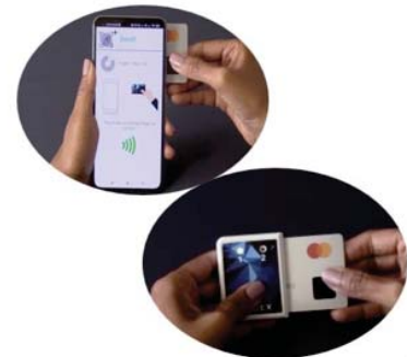
Our enrolment solutions enable the creation of a user fingerprint template, which is encrypted and stored only on the smart card, never in the cloud.
