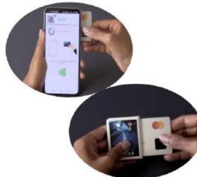
Using one of our proprietary solutions, a user can complete the enrolment process in less than a minute, following simple instructions. Enrollment is completed entirely within the biometric smart card and, importantly, the encrypted fingerprint template is immediately stored only on the card, never in the cloud or on any connected device such as a smart phone or PC.
